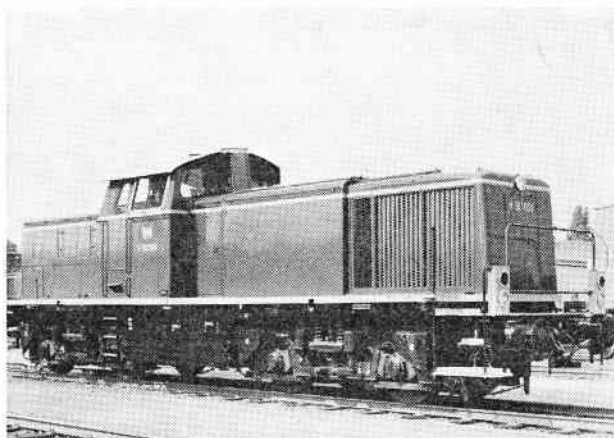
Diesel-hydraulisk rangerloko for tung rangering, V 90.
